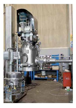
Pressofiltro® agitated Nutsche filters / filter dryers in steam sterilizable design.
