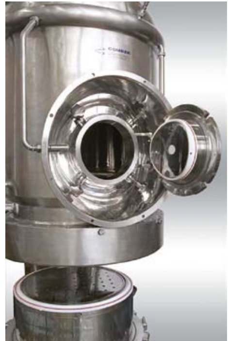
Vessel design for microwaves
