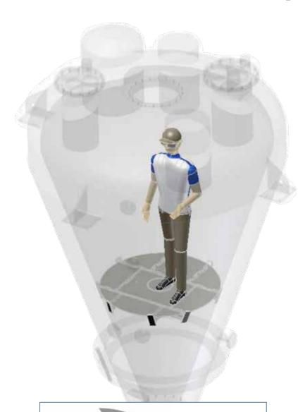
Typical design example: Three modules, each below 30 kg, including diverse customized covers and rubber protections, diameter 1.400 mm
